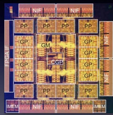
2x2x2 chips in a node 64 cores & 8 pipelines / chip Optical interconnects (~100ns)
